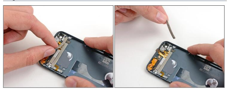
• Peel and remove the foam tape from the rear case of the iPod.
