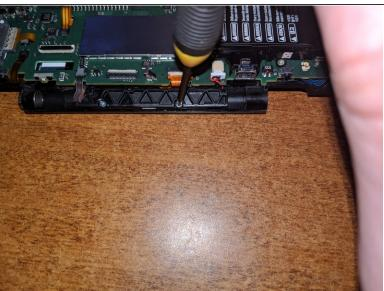
Remove the two screws holding the plastic cover plate down to reveal the red wifi wire which will come out along with the top screen and case.
