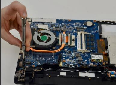
Remove 4 hinge screws with a Phillips #0 screwdriver.
