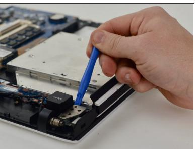
Lift upward on the hinges with a plastic opening tool to release them.
