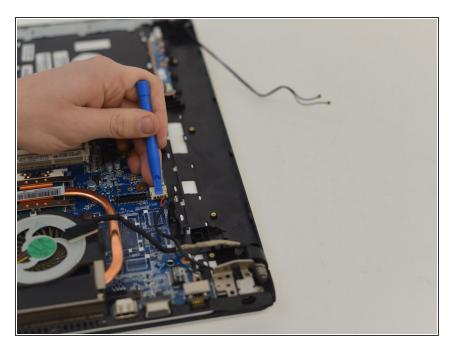
Remove the power display cable with a plastic opening tool by pushing outwards.
