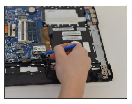
Remove antenna wires attached to the WiFi card using a plastic opening tool.
