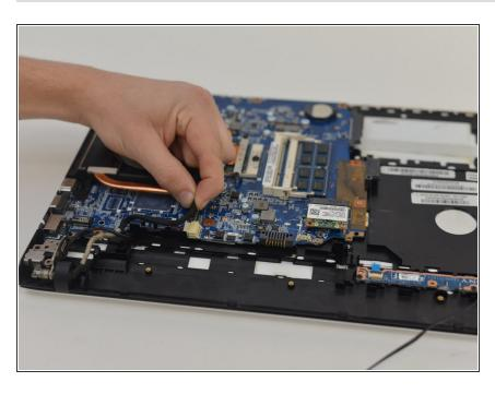
Remove the display cable by pulling upwards.
