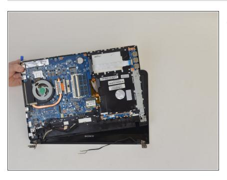
Separate the bottom of the laptop from the monitor.
