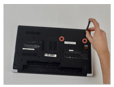
Remove 2 bottom screws in the top right on the HDD cover, with a size P000 screwdriver.
