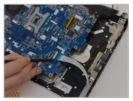
Remove the ribbon cable from the motherboard.
