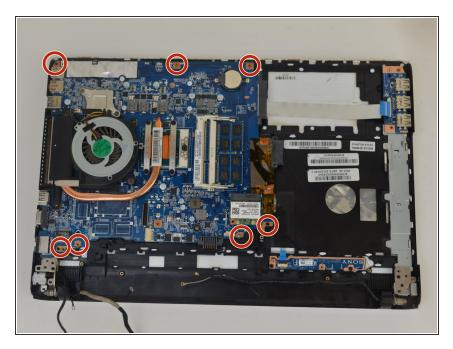
Remove the screws holding the motherboard in place.
