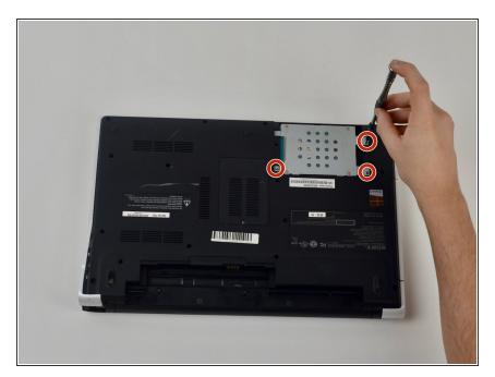
Remove the screws on the HDD with a Phillips #000 screwdriver.
