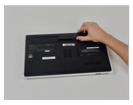
Locate the small gap where the battery and the laptop shell meet.
