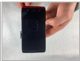
Gently remove SIM card tray from device using a metal spudger.
