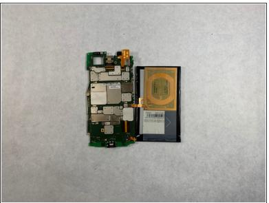
Remove the four T5 Torx screws securing the motherboard.
