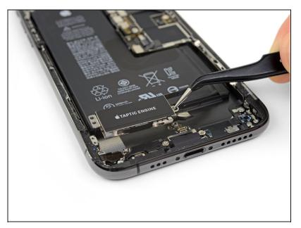
Remove the Taptic Engine assembly.
