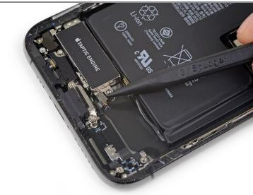
• Use a spudger to disconnect the Taptic Engine flex cable by prying it straight up from its socket.
