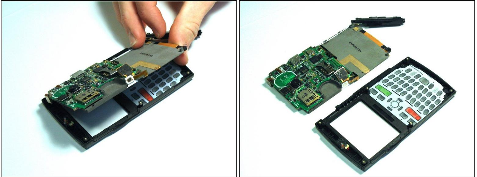
**i** Once all of the connections have been snapped off of the motherboard, the motherboard can be removed.
