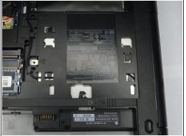
• Remove the Philips PM2.5x6.0 screw that attaches the optical drive to the computer.
