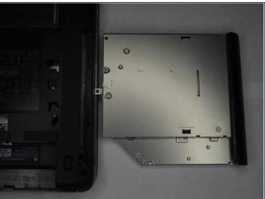
Slowly remove the optical drive, by pulling it straight out of the slot.
