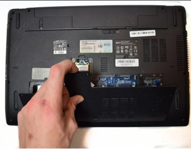
Begin by unscrewing the four phillips #0 7.5mm screws on the plate on the underside. Remove the plate by lifting up.
