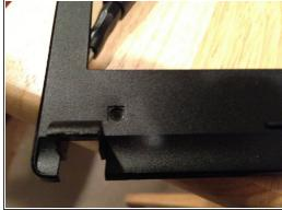
Remove the front bezel using a spudger. The only tricky part here is at the hinges. Tipping the lid backward will reveal the seam on the hinge. Gently separate at the seam and lift the bezel away from the screen
