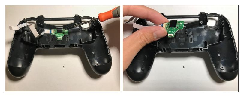
• Unscrew the two screws holding down the USB module.
