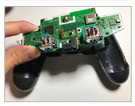
• Remove the second layer PCB. This simply pops out of place.
