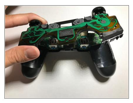
Remove the top layer PCB. The PCB must be popped out of place and then angled in such a way that the trigger buttons at the top of the controller slide out of their slots.
