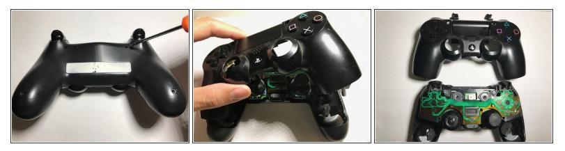
• Begin by removing the screws in the back of the controller.
