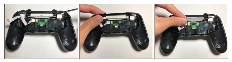
• Unscrew the two screws holding the light assembly together. Once the screws are undone, the parts of the assembly can be pulled out.
