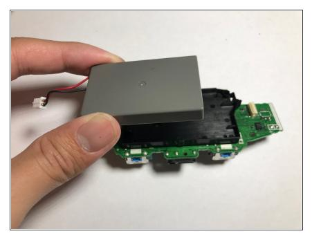
• Flip over the second layer PCB. Remove the battery from its holder.
