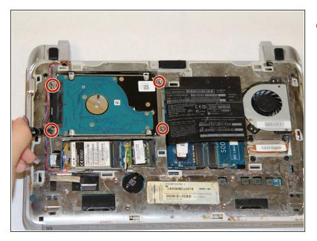
Use your Phillips 0 screwdriver to remove the four 2.5mm Phillips screws which hold the hard drive in place. You can see the 4 screws in the picture circled in red.
