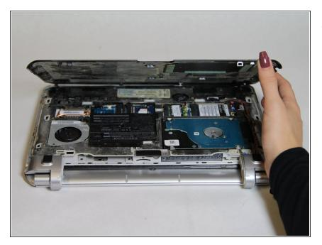
With the battery removed, the back cover can be taken off with your hand.
