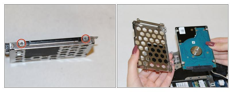
• After removing the enclosure from the device, use your Phillips 0 screwdriver to remove four 3mm Phillips screws. There are two screws on each side of the hard drive enclosure.
