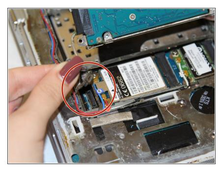
• To disconnect the hard drive from the motherboard, pull the black tab as seen in the picture.
