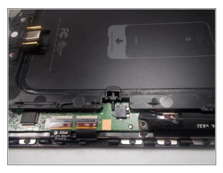
Locate the slider connection.
