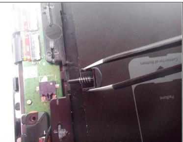
Use tweezers to squeeze and slowly remove the slider connection piece.
