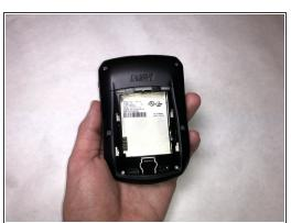
Remove the battery from the compartment.
