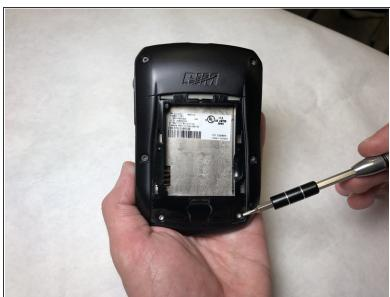
Remove the two 5 mm Torx T6 screws.
