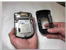
Grab the back housing from the bottom and lift the housing away from you.
