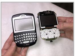
Pull the two pieces apart to separate the front housing from the internals.
