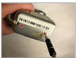
• Unscrew the eight 4mm long JIS #00 screws from the bottom, right side, and the left side.
