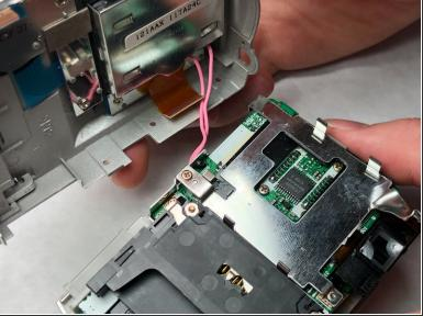
Remove the orange ribbon cable from its connector by firmly but gently pulling it.
