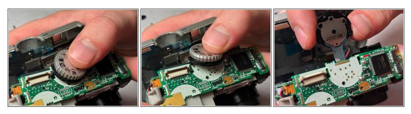
Push or slide the the top dial toward the backside of the camera to unclip from the motherboard.
