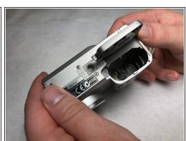
Flip up the cover and remove the battery inside the slot.
