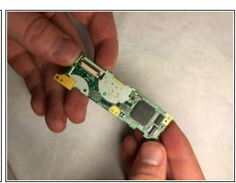
Pull the ribbon connected to the dial off the motherboard.
