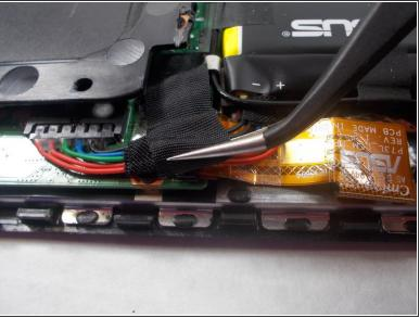
Remove the three pieces of tape that secure the battery and its wires. Peel gently so you don't damage any wires.
