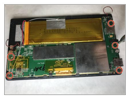
Remove the five 5 mm screws from the motherboard, using the #0 Phillips Screwdriver.
