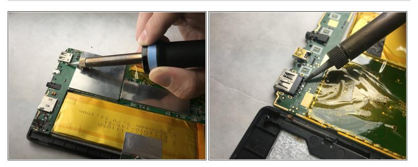
Desolder the eight solder joints holding the USB Port in place.
