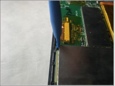
• Using the plastic opening tool tool, pry back the 4 four clips to release the motherboard.
