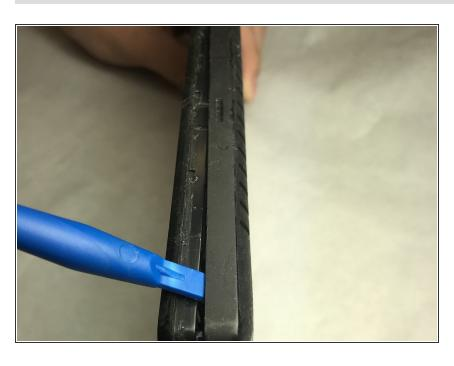
Move the plastic opening tool along the perimeter of the device, loosening the entire back as you go.
