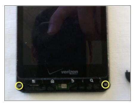
INSTRUCTION: remove the 2 white screws from the lower corners of the screen.
