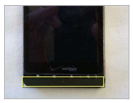
INSTRUCTION: Use the iFixit tool as a crowbar to pry the bottom plastic piece off the phone.
