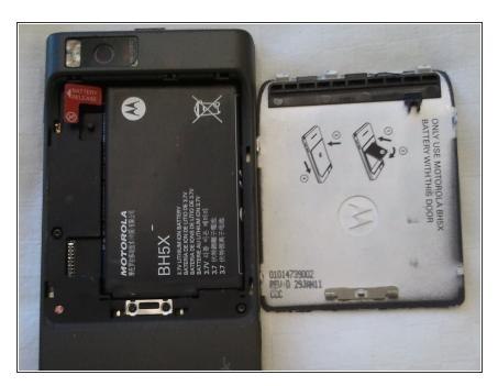
INSTRUCTION: Insert your finger tips into the edges of the opening and pull the casing off.
