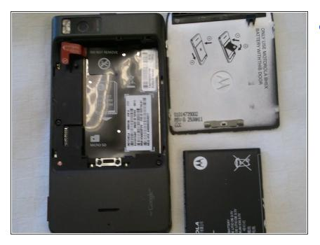
Objective: remove the battery from the battery compartment.
