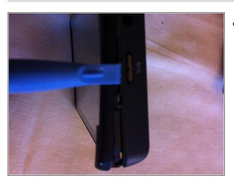
INSTRUCTION: Use the iFixit tool like a crowbar to pry apart the front and rear halves of the casing. They will pop apart.
