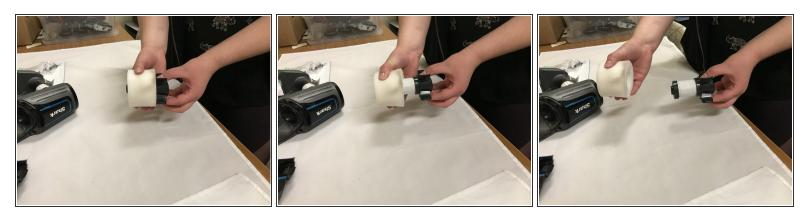
• Grab the larger side of the black plastic ring on the side of the white filter, and separate the white foam filter from the inner filter.
