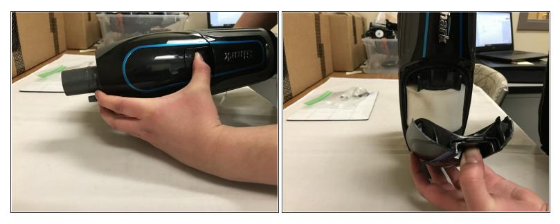
• Squeeze the lever labeled "Clean Filters Monthly" and pull up on the plastic cover.
