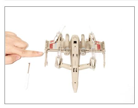
Identify which side gun has broken off.
