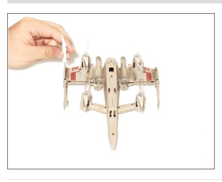
Use the screwdriver to remove the screw holding the side gun in place.
