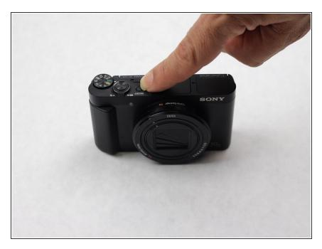
Before disassembling any part of the camera, turn off the power by pressing down on the ON/OFF button. The ON/OFF button is located on top of the camera.
