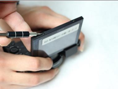
Use the PH000 Phillips head screwdriver to remove the two additional 0.3 mm black Phillips screws located on the top edge of the LCD screen. Place screws on magnetic mat or plastic bag.
