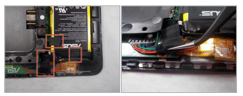
Remove the three pieces of tape that secure the battery and its wires. Peel gently so you don't damage any wires.
