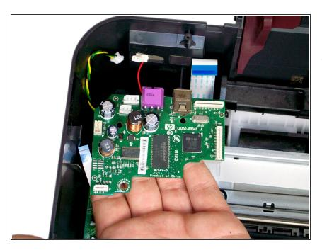
Carefully pull the motherboard out of the printer.
