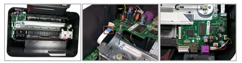
• Turn off the printer then open the top lid in order to see the inside of the printer.
