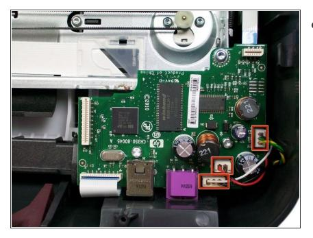
• Locate the three white plugs with wires attached to them. Gently grab the sides of the white chorded plugs and pull them out of their socket.
