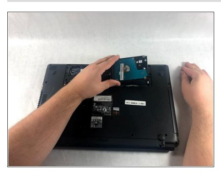
Remove the hard drive from the device.
