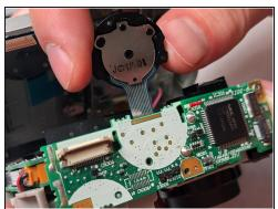
• Push or slide the top dial toward the backside of the camera to unclip from the motherboard.
