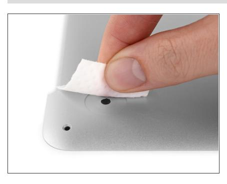
Scrub the foot cavity with adhesive remover to remove any remaining adhesive.
