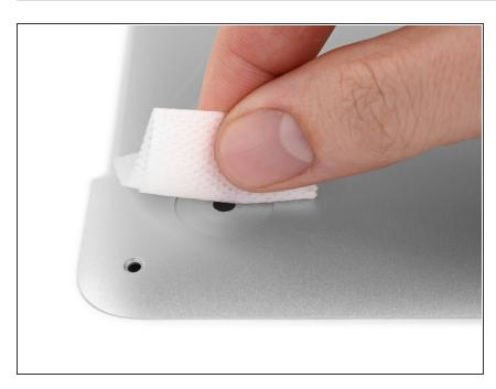
Wipe the foot cavity with an isopropyl alcohol prep pad to remove any cleaner residue and prep the area for the adhesive on the new foot.
