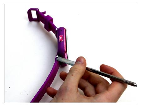
Next, use the flat end of the spudger to wedge between the small-headed pin (located on the band closest to the watch) to pull the pin up through the other side.
