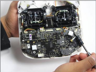
• With the Phillips #00 screwdriver, remove the two Phillips screws.
