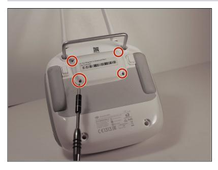
Remove the four screws with a Torx T8 screwdriver to access the back con board.
