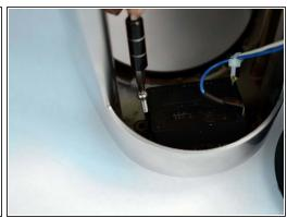
Remove two 11.59mm T10 screws.
