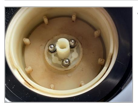
This is the correct position of bearings and springs when the screw and bottom burr are removed.
