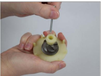
Remove the loosened screw by pulling it upwards.
