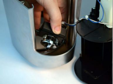
Remove the time/on switch by pulling upwards.
