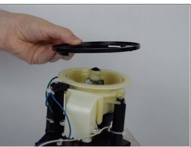
Grab the edge of the plastic black ring that sits on top of the device and gently pull up to release.
