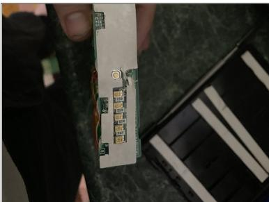
Battery connector on PCB
