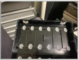
Top of battery pack with upper case removed. Case is NOT glued on, but is clipped on. You can see the case clips (and damaged top retention areas) from where I pulled it apart.
