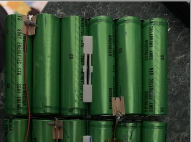
Wiring. Three leads for balance charging., red and black are for the 14.8v connections. The pack is separated into 4 sets of 3 cells each run in series.
