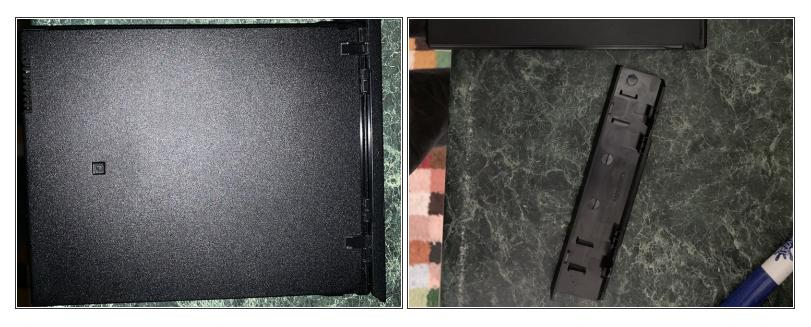
Underside of battery, as you can see the slide part comes off. the slide part is there to adjust for if the battery is on the left or right bay of the laptop.
