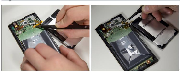
• Use the <u>tweezers</u> to remove the Pancake connector that connects the battery to the phone.
