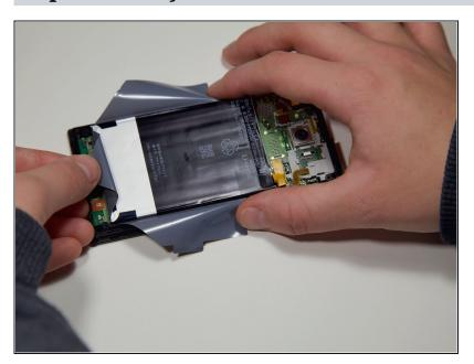
Peel back the grey paper wrapping around the battery.
