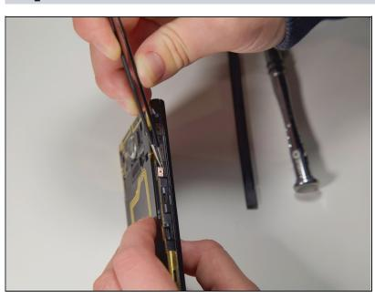
Use the <u>tweezers</u> to remove the pink clips on either side of the device and then take the casing off.
