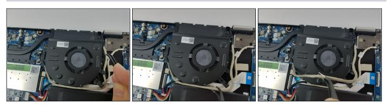
• Using the Precision Tweezers, remove the 2 gray wires around the fan from their clips.
