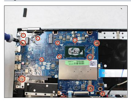
Unscrew the twelve 4mm screws with a #0 Phillips screwdriver.
