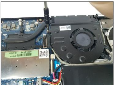
• Remove the two 4 mm Phillips #0 screws which mount the fan.
