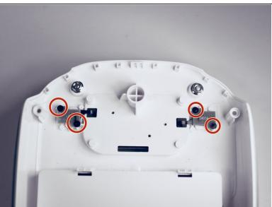
Using a Phillips #00 screwdriver, remove the four screws on the inside of the panel. That will allow you to remove the buttons by gently lifting them with your hands.
