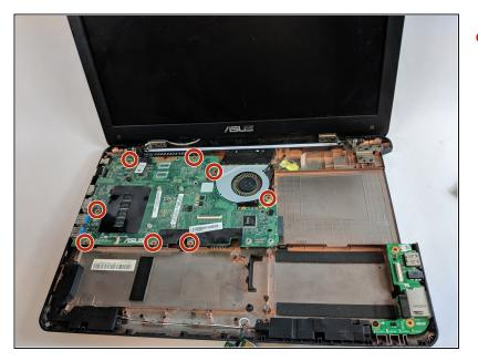
Remove the eight 5.7mm screws using the Phillips #0 Screwdriver.
