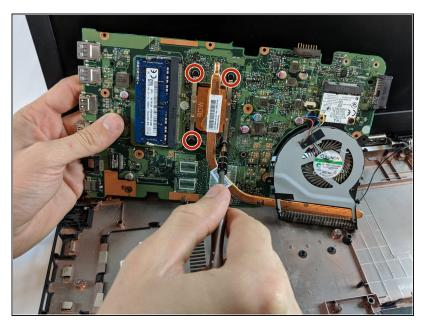
Unscrew and remove the four 0.01mm screws using the Phillips #0 Screwdriver from the heatsink.
