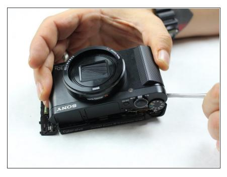
After loosening the plastic edges of the camera, gently pull the LCD screen side upwards.
