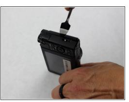
Use the plastic opening tools included in the iFixit tool kit first. If the shell/parts do not detach
