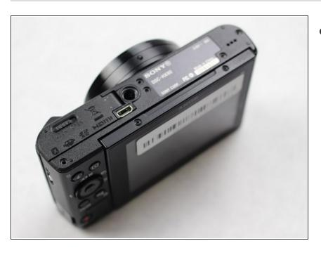
Do not remove the screws holding the LCD screen together.
