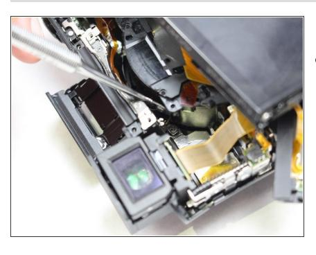
Use metal spudger to detach top part off the rest of the camera. Be extremely careful as there is a thin golden film/plastic ribbon holding the top piece to the rest of the camera.
