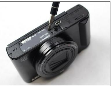
Use the PH000 Phillips head screwdriver (from iFixit tool kit) to take the screws out. Begin unscrewing from the bottom of camera. At the end of this step there will be a total of five black 0.4 mm Phillips screws. Place them on a magnetic mat or a plastic bag.
