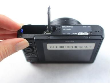
Open the compartment located at the bottom of the camera. Slide the LOCK/OPEN switch to the OPEN side. Locate the small blue tab on the side. Pull it in direction away from the battery.
