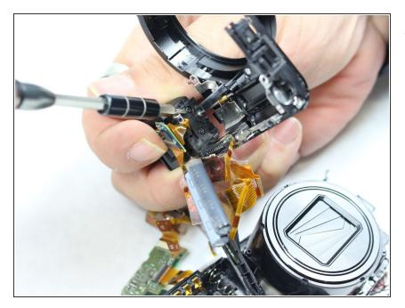
After removing circuit board, find two 0.3 mm black Phillips screws located at the bottom of viewfinder. Remove the screws with PH000 Phillips head screwdriver. Place the screws on magnetic mat or plastic bag.
