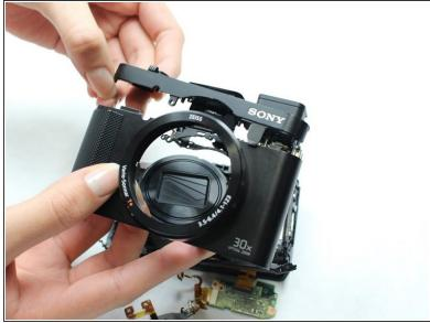
Gently pull the circuit board off the top piece of the camera. The top piece will be detached from the rest of the camera. Removing the top of the camera will make it easier to access the viewfinder.
