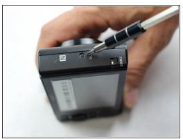
Keep working alongside the edge of camera until no screws are left in place. In addition to the five screws from the bottom, there will be a total of three more 0.4 mm black Phillips screws. Place them on the magnetic mat or plastic bag.
