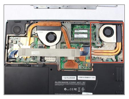
Once the cover has been removed, locate the CPU Cooler to begin the replacement.
