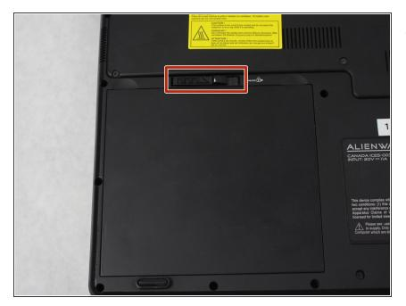
Push the slider until the battery is released from its socket.
