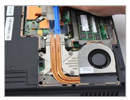
Once all screws have been removed and the cooler has been unplugged, gently lift the cooler out of its compartment to install the new cooling fan.
