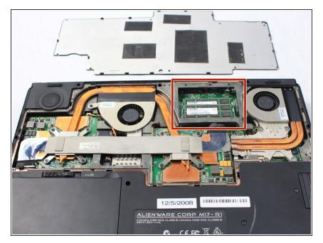
Once the cover is removed, locate the RAM compartment to begin the replacement.
