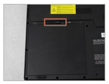
Push the slider until the battery is released from its socket.
