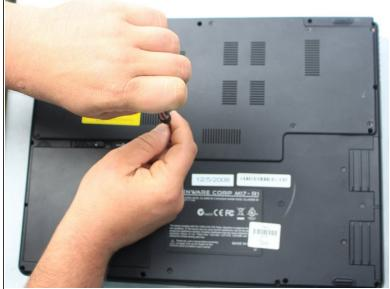
• Remove the nine 3 mm screws that secure the cover using a Phillips #1 screwdriver.
