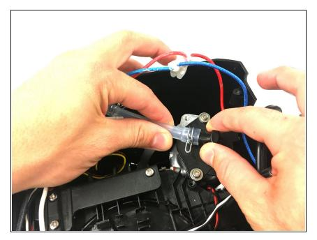
Detach the valve tubes from the device by pinching the pins and sliding the valve tubes off.
