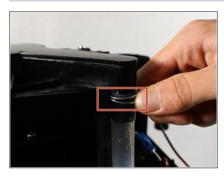
Separate hose from upper nozzle by squeezing the clamp and pulling the hose down slightly.
