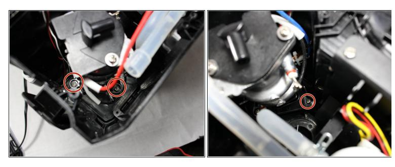
Using a #1 Phillips head screwdriver with an extension, remove three 6mm screws holding the heater to the unit.
