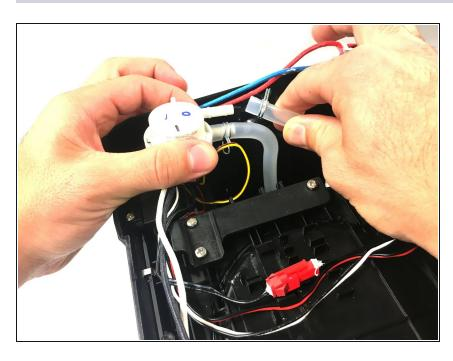
Detach the valve tubes from the valve by squeezing the pins and pulling them away from the valve.
