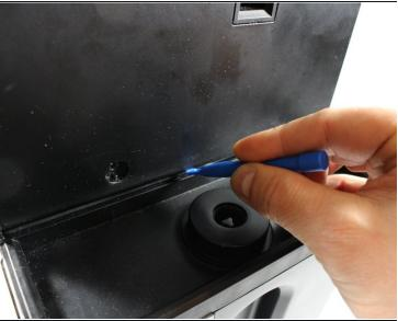
Slowly pry the upper cover away from the unit on top of the brew basket, and near the base of the water reservoir along the side of the upper cover.
