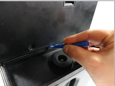
Gently pry the upper cover off the unit above the brew basket and above the water reservoir base and along the side of the upper cover.
