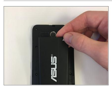
Lift the battery out from the top of the device.
