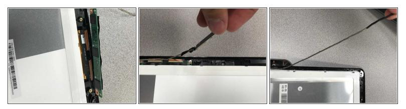
• Slowly pull up the webcam out of its slot, and begin to remove the wire.
