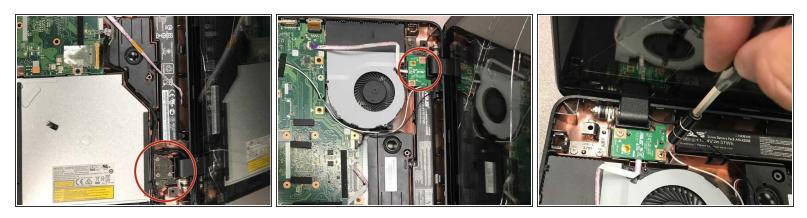
• Remove eight 4.4 Phillips #00 screws attached to the hinge.
