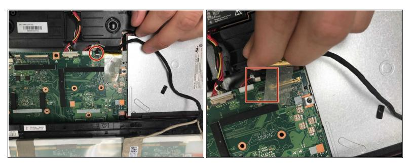
Once the sticker is peeled off pull the plug holding the webcam into the circuit board and the webcam is now disconnected.
