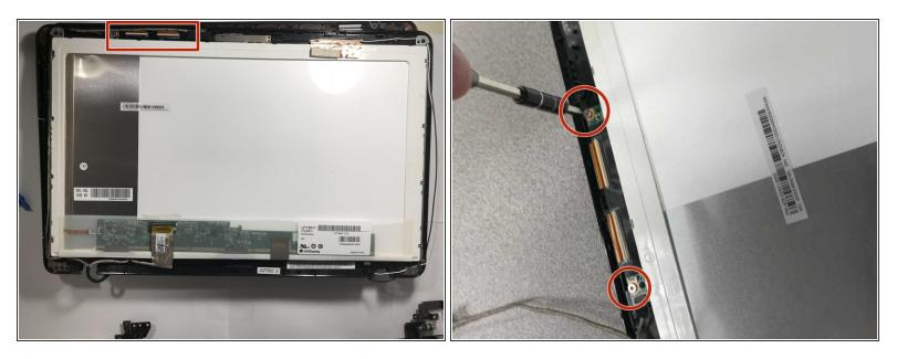
Remove the two 4mm Phillips #00 screws attached to the webcam.
