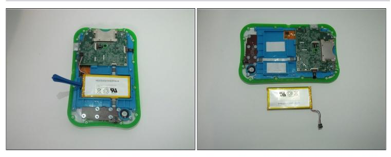
• Carefully remove the battery from the LeapPad. Use an opening tool or a plastic spudger to gain leverage, if needed.
