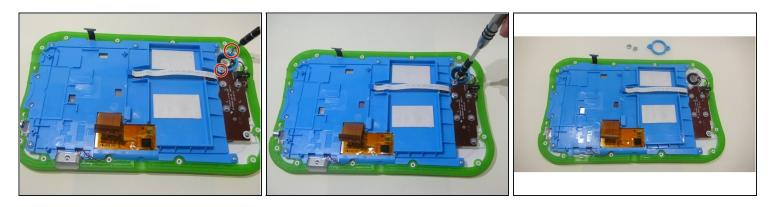
• Remove the circular plastic speaker and the 2 screws a Phillips #1 screwdriver. Gently lift the cover off of the device.
