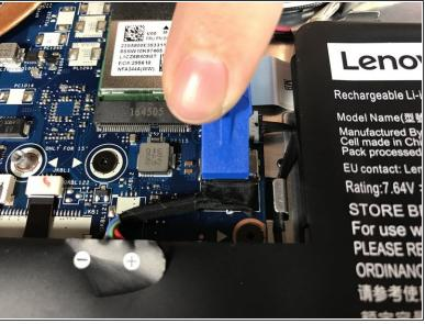
• Use your fingers or an opening tool to slide the battery connector out of its motherboard socket.
