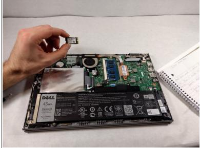
• Using your fingers, pull the WLAN card up and away from the device.
