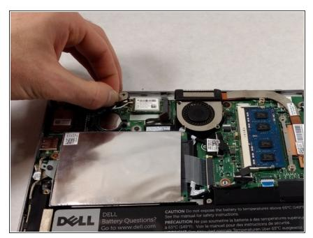
Remove the two wires by pulling them upward, away from the WLAN card.
