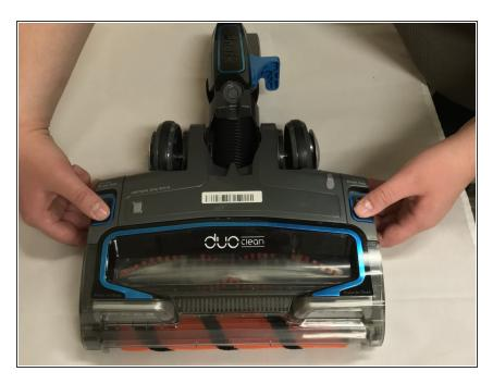
Press and slide the access brush roll buttons towards the "Access Brush Roll" printing on casing.
