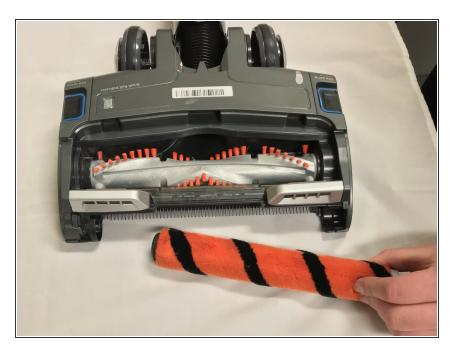
Pull the red Pull tab that is located on the right side of the soft brush roll away from the front of the vacuum and place the soft brush roll to the side.
