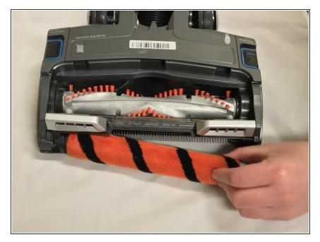
Lift plastic casing upward and off of the top of the floor unit. Place off to the side.
