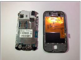
Disconnect the orange motherboard connection, then remove interior hardware from the front screen display.
