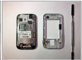
Use metal pry tool to separate the interior back panel from the interior hardware and screen.
