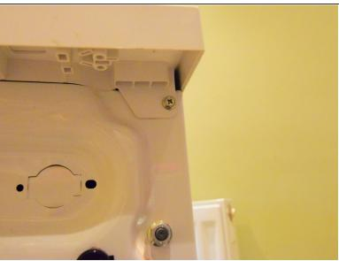
The top lid is held in place with two screws at the back as indicated. Remove these, and lift the lid off
