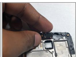
Lastly, take out the ear piece out of its housing using a plastic pry tool.
