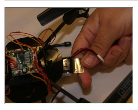
Remove the battery from the slot by pulling on the silver tab attached to the exposed end of the battery.
