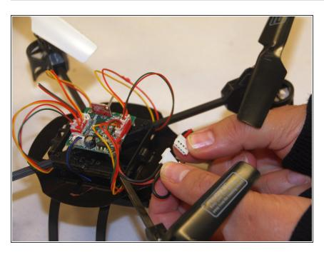
Disconnect the battery from the drone by separating the red and black battery cable from the red and black drone cable.
