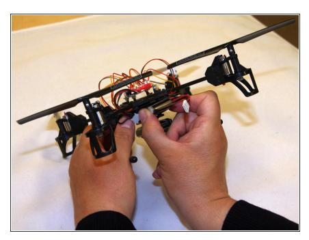
Locate the drone battery housed in the slot between the drone body and the camera.
