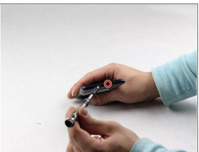
Using a removable head screwdriver and a T3 bit, begin by removing the two screws located on either side of the charging port.
