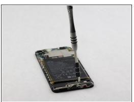
Once the back has been removed, you will need to unscrew the four screws on the bottom panel with an AT3 bit.
