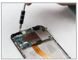
Using the screwdriver with the PH0 bit, unscrew all screws found on the circuit board.
