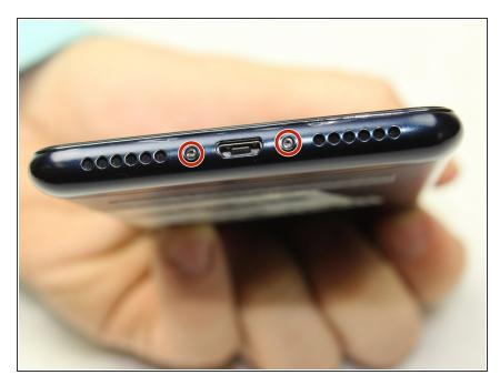
Using a removable head screwdriver and a T4 bit, remove the screws on the base of the phone on either side of the charging port.
