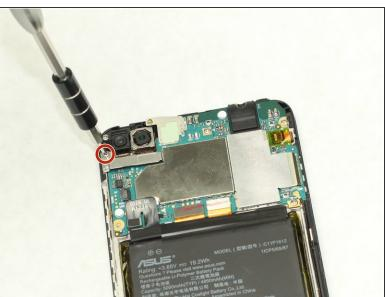
Using a removable head screwdriver and a PH0 bit, begin removing the panel beneath the two cameras by unscrewing the screw.
