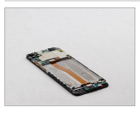
Remove the battery and replace it with the new battery.
