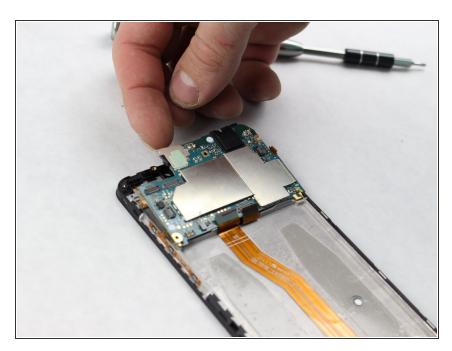
Gently lift and remove the circuit board.
